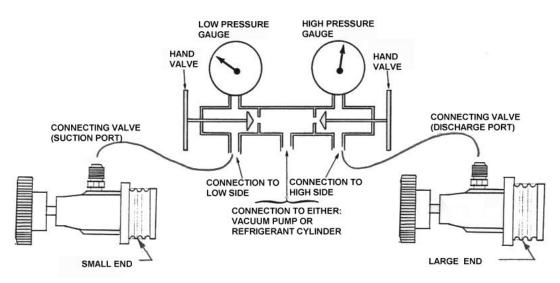
Gauges are used in the evacuation and charging. They will provide information on the operation of the system.
